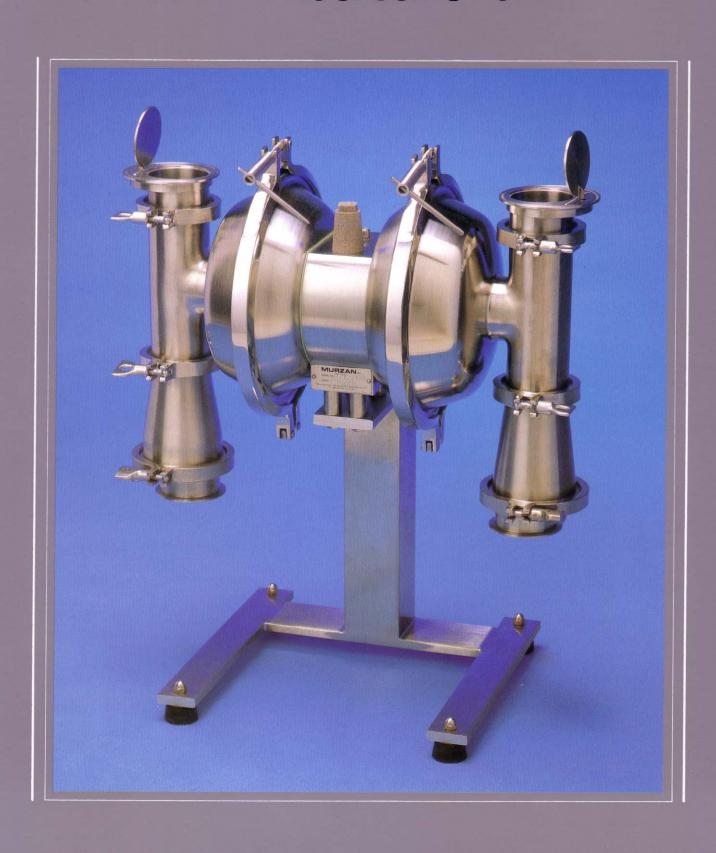
The Murzan PI 50 is the only sanitary diaphragm pump specifically designed with the needs of the poultry industry in mind. This pump can easily handle solids up to 6" (15 cm) in diameter or 7" (17 cm) long without damaging the product - suitable for pumping necks, gizzards, livers, hearts, feet, blood, or any other application in a poultry processing plant. The Murzan PI 50 is FDA approved and USDA Meat & Poultry listed.
