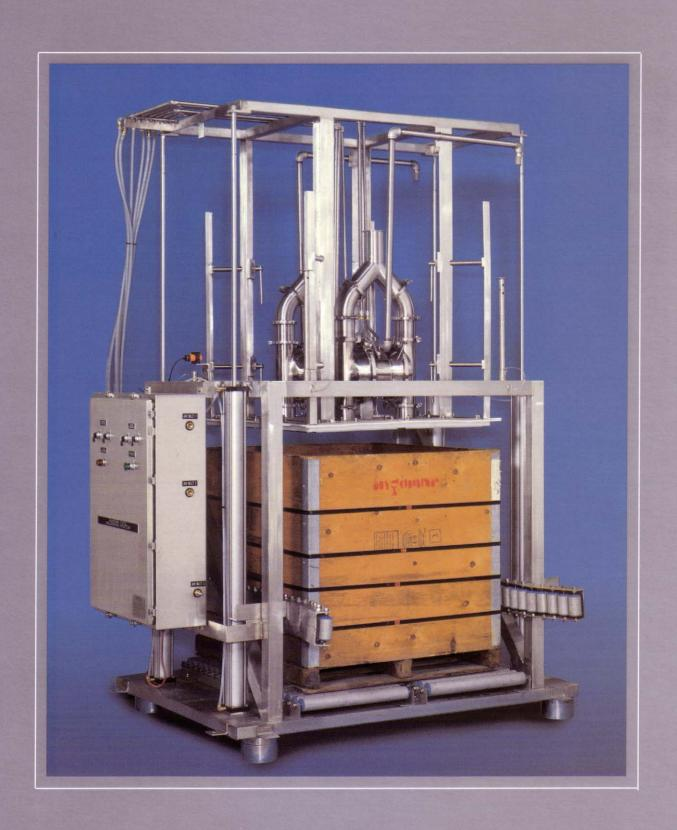
The Murzan TUS-50 is the ideal solution for emptying up to 300 gallon containers of highly viscous, and/or heavy materials, applications which no pump alone can handle. This system quickly empties and cleans TOMATO PASTE containers without putting any pressure on the product or the container.
